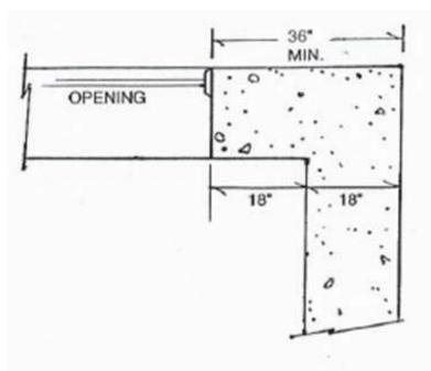
THE MINIMUM DISTANCE MEASURED FROM THE EDGE OF ANY OPENING TO THE NEAREST CORNER, PLUS THE ADJOINING WALL THICKNESS SHALL NOT BE LESS THAN 36 INCHES
